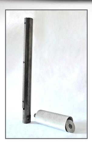
Walt Powley Inline's exclusive design mini rotary plow assembly. Custom engineered and manufactured to assist in the making of smaller plow folds.
